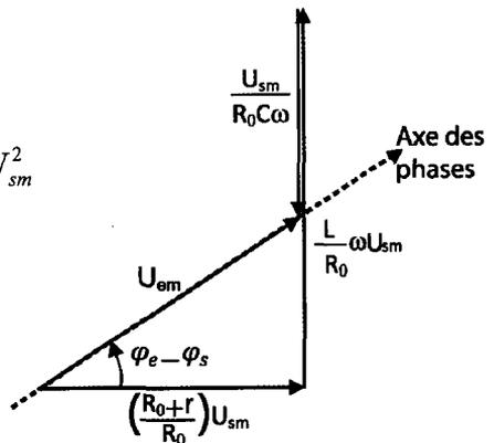
$$\frac{U_{sm}}{U_m} = \frac{1}{\sqrt{\left(\frac{R}{R_o}\right)^2 + \left(\frac{L\omega}{R_o} - \frac{1}{R_o c\omega}\right)^2}} = \frac{R_o}{R} \frac{1}{\sqrt{1 + \left(\frac{L\omega}{R} - \frac{1}{Rc\omega}\right)^2}}$$
