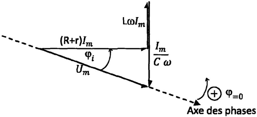
$$\alpha * U_m^2 = (R+r)^2 I_m^2 + (L\omega I_m - \frac{I_m}{C\omega})^2$$
