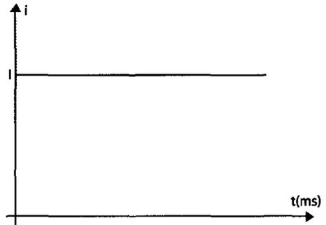
$$2) u_c = \frac{q}{C} = \frac{It_1}{C} \Rightarrow t_1 = \frac{C \cdot u_c}{I} ; AN t_1 = \frac{2 \cdot 10^{-6} \times 10}{10^{-3}} = 210^{-2} s$$
