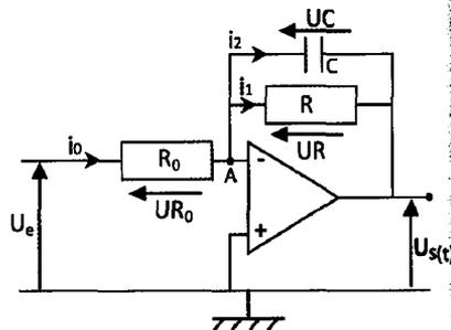
$$i_0 = \frac{u_{R_0}}{R_0} \text{ or } u_{R_0} = u_e \Rightarrow i_0 = \frac{u_e}{R_0}$$
