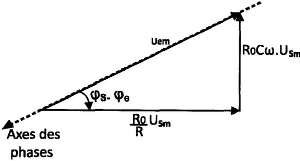
$$U_{Cm}^2 = \left( \frac{R_0}{R} U_{Sm} \right)^2 + (R_0 C \omega U_{sm})^2 = U_{sm} \left[ \left( \frac{R_0}{R} \right)^2 + (R_0 C \omega)^2 \right]$$
