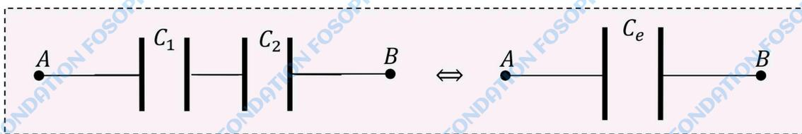
$$U_{AB} = U_1 + U_2 = Q \left( \frac{1}{C_1} + \frac{1}{C_2} \right) = \frac{Q}{C_e} \Rightarrow$$
