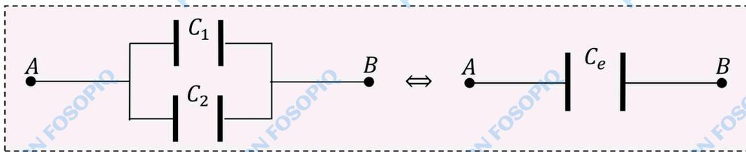
$$Q_1 = C_1 U_{AB} \text{ et } Q_2 = C_2 U_{AB} \Rightarrow Q_1 + Q_2 = (C_1 + C_2) U_{AB} \text{ or } Q_t = Q_1 + Q_2 = C_e U_{AB}$$
